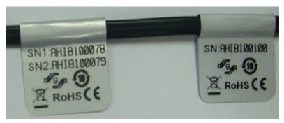
A DPX2, DPX3, DX or DX2 sensor package has a serial number tag attached to its rear side.
