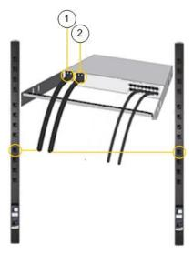
1. Use the power cords that came with KX III. Use both cords with AC power outlets for dual-power failover protection.
