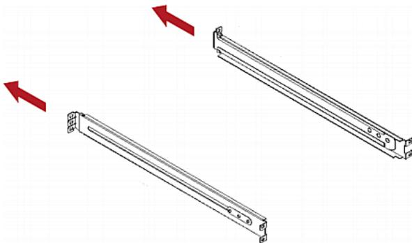
2. Fasten the brackets to the rack rails securely with your own fasteners.
