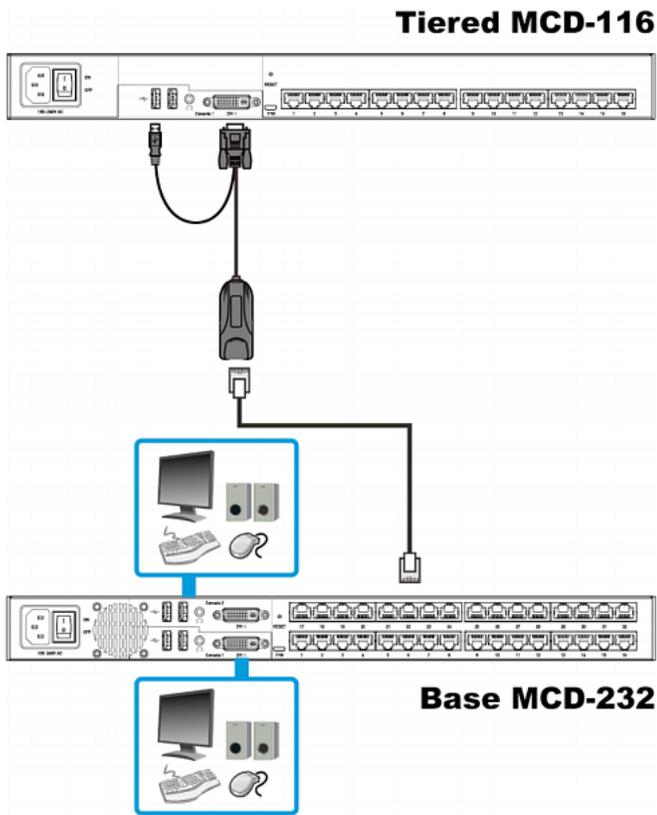
Warning: If any 2nd-tier switch is a dual-user MCD model, DO NOT connect a keyboard, mouse and monitor to Console 2 because Console 2 is disabled.
