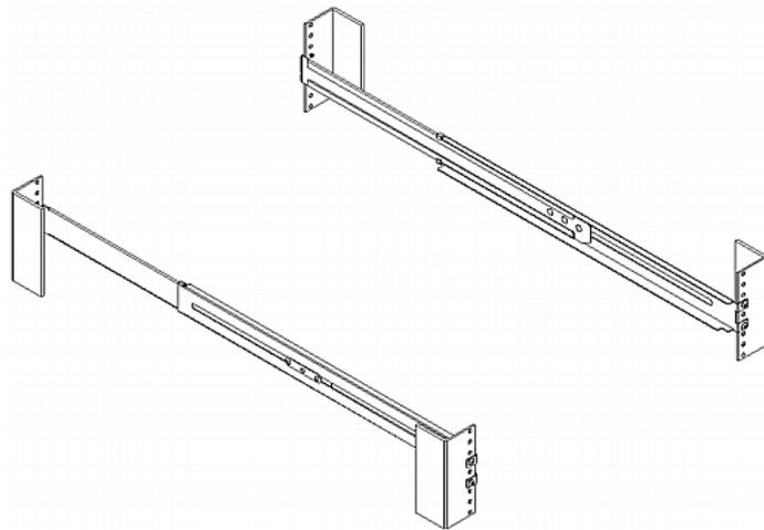
3. Slide the MCD-LED between the brackets.
