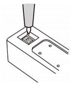
5. To set the Normal state for channel 2, repeat Step 4 for adjusting the other dip switch's setting.
