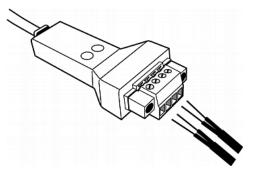
3. Use a screwdriver with a 2.5 mm wide shaft to tighten the screws above each termination point to secure the wires, using a torque of 0.196 N·m (2 kgf·cm).
