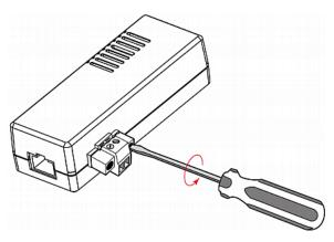
2. Separate the terminal module from the sensor box.
