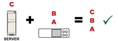
In reality some servers may provide a partial (or even a full) certificate chain instead of a single server certificate. If your server provides a partial certificate chain containing 'Certificate B' and 'Certificate C', then you only need to upload 'Certificate A" to the receiver. If the server has a full certificate chain containing Certificates 'A', 'B', and 'C', then you also need to upload the root certificate 'A".
