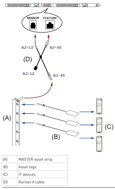
Tip: To connect Raritan's environmental sensor packages to PX2, connect them to the female RJ-12 connector of the X cable. For details, see Using an X Cable (on page 63).
