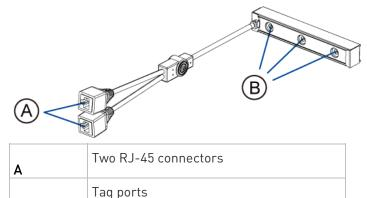
Important: DO NOT hot swap or hot plug any AMS-Mx-Z in a composite asset strip chain after connecting the chain to the PX2 device. Doing so may cause the device's FEATURE port to malfunction.
