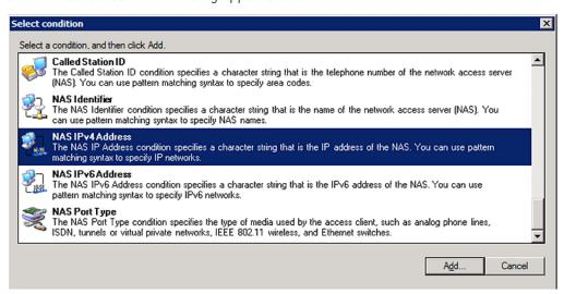
6. The NAS IPv4 Address dialog appears. Type the PX2 IP address -- *192.168.56.29*, and click OK.
