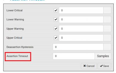
In the threshold settings, the Assertion Timeout field postpones the "assertion" action. It determines how long a sensor must remain in the "worse" new state before the PX2 triggers the "assertion" action. If that sensor changes its state again within the specified wait time, the PX2 does NOT assert the worse state.
