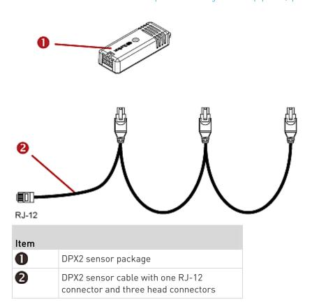
The following procedure illustrates a DPX2 sensor cable with three head connectors. Your sensor cable may have fewer head connectors.
