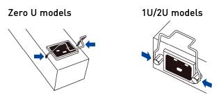
Connect the power cord to the inlet, and press the clip to hold the cord.
