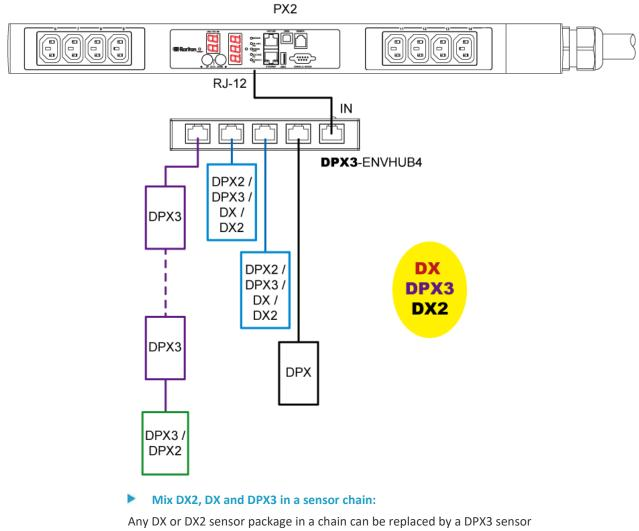
Any DX or DX2 sensor package in a chain can be replaced by a DPX3 sensor package, or vice versa. The total number of sensor packages in this chain cannot exceed 12.
