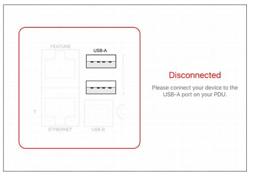
A diagram in PDView indicates the appropriate USB port your mobile device should connect according to your mobile operating system.
