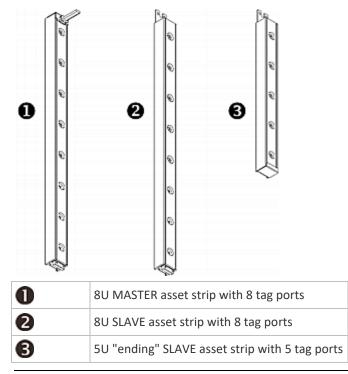
Note: Unlike general slave asset strips, which have one DIN connector respectively on either end, the ending slave asset strip has one DIN connector on only one end. An ending asset strip is installed at the end of the asset strip assembly.
