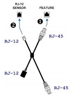
3. Plug the male RJ-45 connector at the longer end of the X cable into the RJ-45 port labeled "Input" on the composite asset strips.
