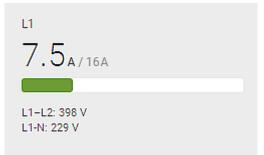
The right side shows the current and voltage data per phase. For a single-phase device, it shows only one line, but for a three-phase device, it shows three lines (L1, L2 and L3).
