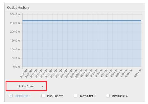
Available data types include RMS current, RMS voltage, active power and apparent power.
