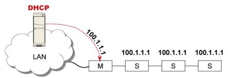
In this mode, the DHCP server communicates with the master device alone and assigns one IP address to the master device. All slave devices share the same IP address as the master device.
