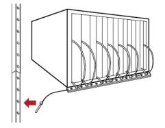
6. Repeat the above steps to connect additional blade extension strips. Up to 128 asset tags on blade extension strips are supported per FEATURE port.
