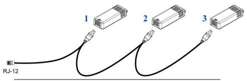
Tip: If the number of sensors you are connecting is less than the number of head connectors on your sensor cable, connect them to the first one or first two head connectors to ensure that there are NO free head connectors prior to the final DPX2 sensor package attached.
