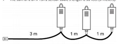
The sum of a DPX-T3H1 sensor cable's length is 16 feet (5 meters).
