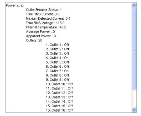
2. A status box appears, displaying details of the controlled PX2, including power state of each outlet on the device.
