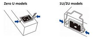
3. Connect the power cord to the inlet, and press the clip toward the power cord until it holds the cord firmly.
