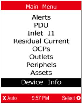
The image shows a point matrix LCD screen with a red header bar at the top containing the text "Main Menu". The main menu items are listed in the center: Alerts, PDU, Inlet I1, Residual Current, OCPs, Outlets, Periphels, and Assets. At the bottom, there is a black bar with "Device Info" in white. Below the screen, a status bar is highlighted in red, showing "X Auto", "9:57 PM", and "Select" with a right-pointing arrow. |
