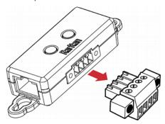
3. After connecting detectors/switches to the terminal module, plug the terminal module back into the sensor box, and then tighten the screws at two sides of the terminal module.
