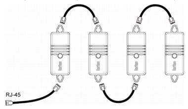
3. Make sure the total number of cascaded sensors does not exceed 32 per sensor port. See *Supported Maximum Number of Sensors and Actuators* (on page 78).
