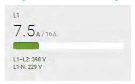
The right side shows the current and voltage data per phase. For a single-phase device, it shows only one line, but for a three-phase device, it shows three lines (L1, L2 and L3).
