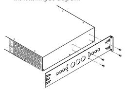
2. Insert the cable-support bar into rackmount brackets.
