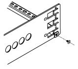
4. On a 2U model, repeat the above steps to install another cable-support bar.
