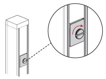
Repeat the same steps to install the other button onto the PDU's rear side.
