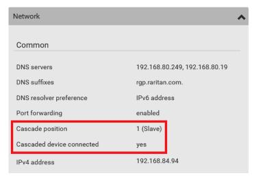
The final slave device shows a non-zero number which indicates its position in the 'Cascade position' field and no in the 'Cascaded device connected' field.
