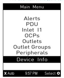
If any alerts exist, the top and bottom bars on the LCD display change the color from black to yellow or red. See *Operating the Dot-Matrix LCD Display* (on page 68).
