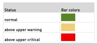
Note: The "below lower warning" and "below lower critical" states also show yellow and red colors respectively. However, it is not meaningful to enable the two thresholds for current levels.
