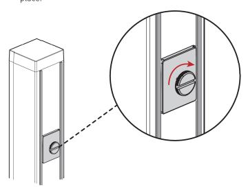
Repeat the same steps to install the other button onto the PDU's rear side.
