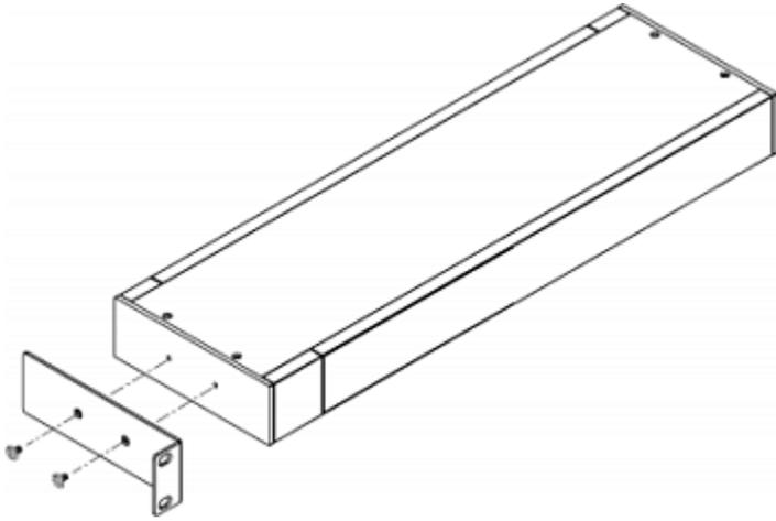
2. Attach PXC to the rack. Fasten the rackmount brackets' ears to the rack using your own fasteners.
