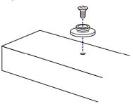
4. Press the PDU forward, pushing the mounting buttons through the mounting holes, then letting the PDU drop slightly.
