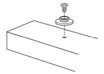
4. Press the PDU forward, pushing the mounting buttons through the mounting holes, then letting the PDU drop slightly.
