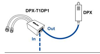
*Note: You CANNOT cascade more than two sensor packages in this DPX sensor chain.*
