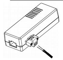
3. Use a screwdriver with a 2.5 mm wide shaft to tighten the screws above each termination point to secure the wires, using a torque of 0.196 N·m (2 kgf·cm).
