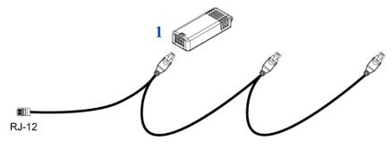
• Scenario B: When only two sensors are connected, always connect them to the first two head connectors.
