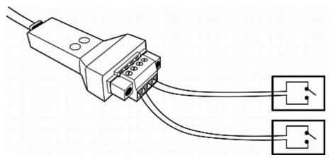
For details on connecting a detector/switch, see *Connecting Detectors/Switches to DPX-CC2-TR* (on page 60).
