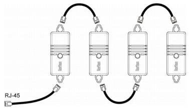
Make sure the total number of cascaded sensors does not exceed 32 per sensor port. See *Supported Maximum Number of Sensors and Actuators* (on page 78).
