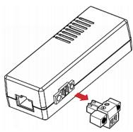
3. After connecting detectors/switches to the terminal module, plug the terminal module back into the sensor box, and then tighten the screws at two sides of the terminal module.
