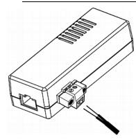
3. Use a screwdriver with a 2.5 mm wide shaft to tighten the screws above each termination point to secure the wires, using a torque of 0.196 N·m (2 kgf·cm).
