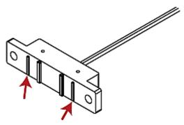
When there is some water between the two poles, it causes current loop back on the water sensor to trigger the alarm.
