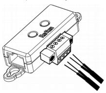
3. Use a screwdriver with a 2.5 mm wide shaft to tighten the screws above each termination point to secure the wires, using a torque of 0.196 N⋅m (2 kgf⋅cm).
