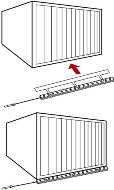
3. Connect one end of an asset tag to a blade server and the other end to the blade extension strip.
