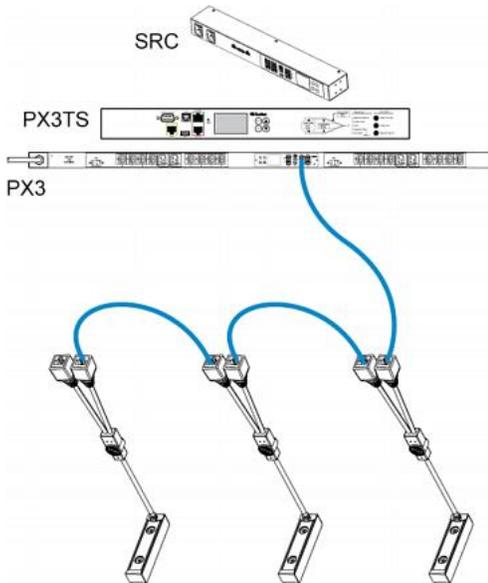
5. Repeat Step 3 to connect IT devices to the other composite asset strips in the chain.
