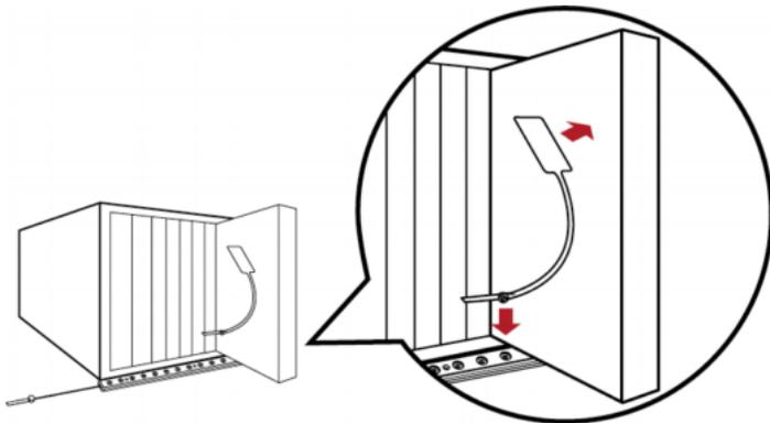
4. Repeat the above step until all blade servers in the chassis are connected to the blade extension strip via asset tags.
