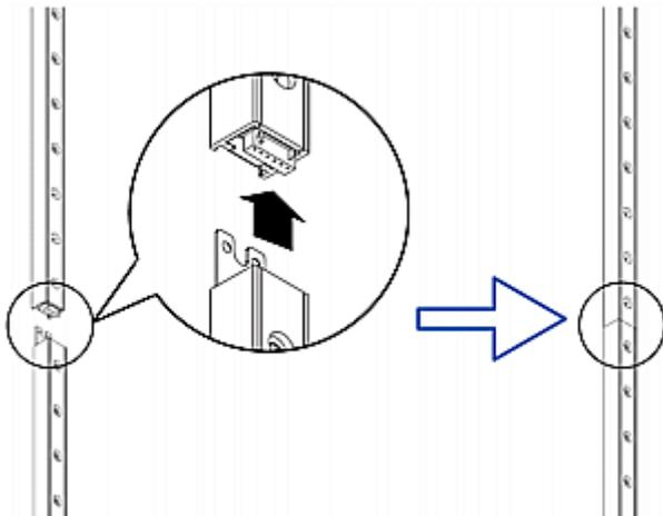
2. Connect another slave strip to the one being attached to the master strip in the same manner as Step 1.
