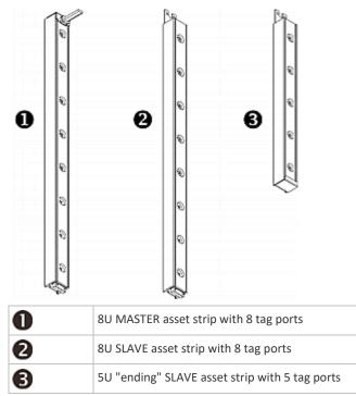
Note: Unlike general slave asset strips, which have one DIN connector respectively on either end, the ending slave asset strip has one DIN connector on only one end. An ending asset strip is installed at the end of the asset strip assembly.
