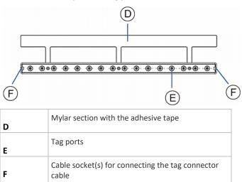
Note: Each tag port on the blade extension strip is labeled a number, which is displayed as the slot number in the Raritan Asset Management Gateway device's web interface.
