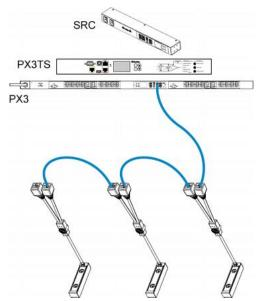
5. Repeat Step 3 to connect IT devices to the other composite asset strips in the chain.
