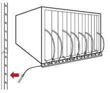
Repeat the above steps to connect additional blade extension strips. Up to 128 asset tags on blade extension strips are supported per FEATURE port.
