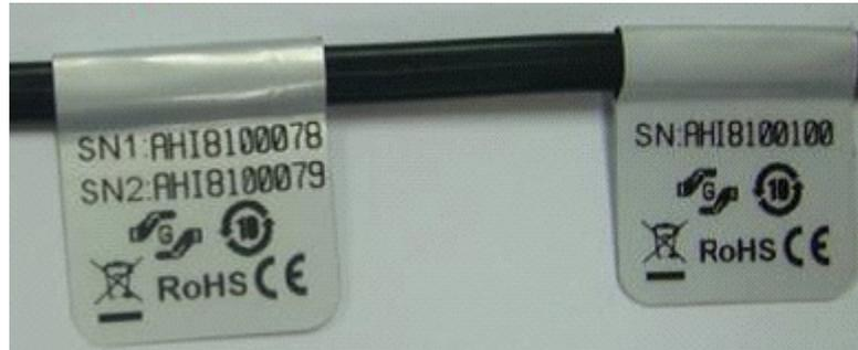
A DPX2, DPX3, DX or DX2 sensor package has a serial number tag attached to its rear side.
