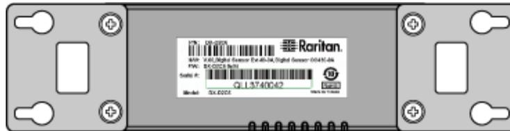
The serial number for each sensor or actuator appears listed in the web interface after each sensor or actuator is detected by the BCM2. Match the serial number from the tag to those listed in the sensor table.
