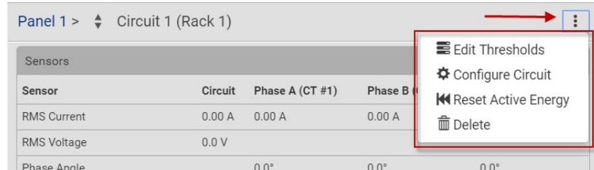
The screenshot shows the "Circuit 1 (Rack 1)" details page. The breadcrumb is "Panel 1 > Circuit 1 (Rack 1)". A table of sensors is visible, and an actions menu is open in the top right corner, showing options: "Edit Thresholds", "Configure Circuit", "Reset Active Energy", and "Delete". A red arrow points from the menu to the top right corner.
