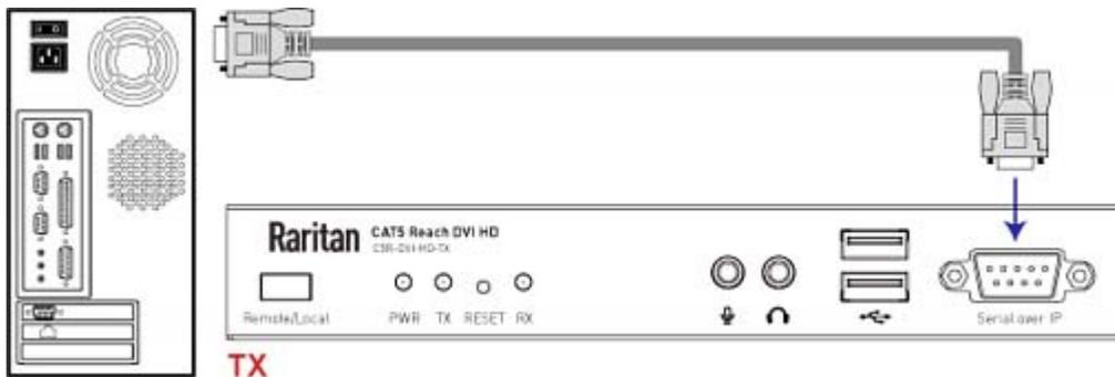
3. Connect an RS-232 cable between the receiver's "Serial over IP" port and the Raritan PDU's RS-232 port.
