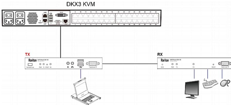
► **To extend the distance between two tiered KVM switches:**
