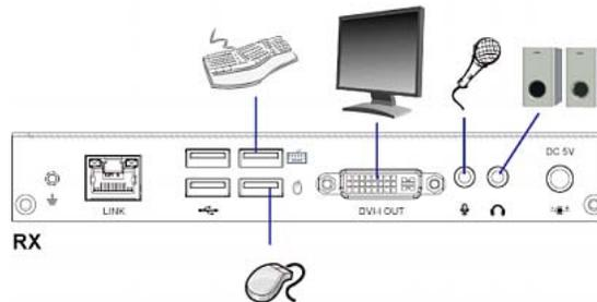
4. Use a Cat5e/6 cable up to 330 feet (100 meters) long to connect the transmitter and receiver. Plug either end of the cable into the RJ-45 LINK ports.
