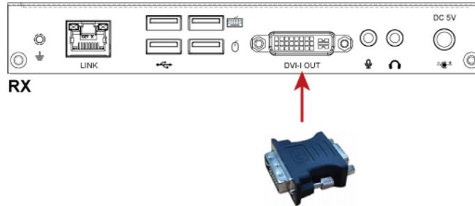
*Note: In case you have used two DVI-I to VGA adapters on the transmitter, you need to purchase one more from Raritan if you will connect a VGA monitor to the receiver.*
