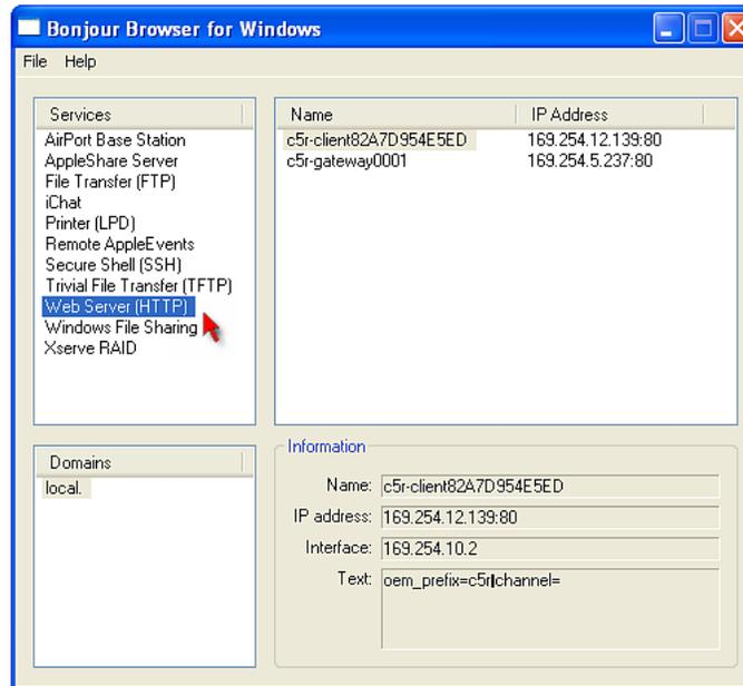
4. Launch the web browser, and type the transmitter's IP address. The transmitter's web user interface displays.
