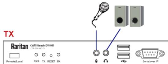
3. Connect the speakers and microphone to the Audio Out and Microphone In jacks of the receiver.
