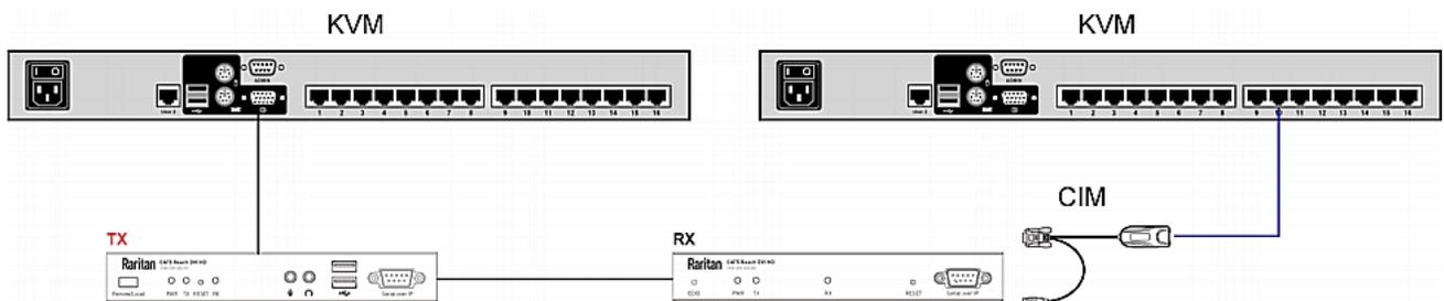
► **To extend the distance between any computer and a KVM switch:**
