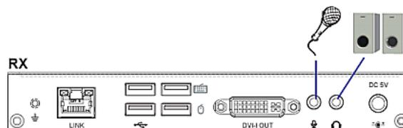
4. Use a Cat5e/6 cable up to 330 feet (100 meters) long to connect the transmitter and receiver. Plug either end of the cable into the RJ-45 LINK ports.
