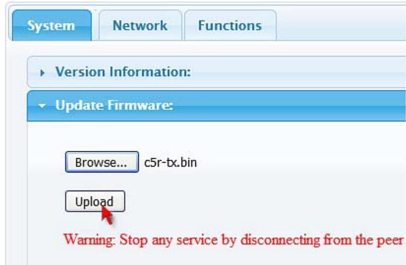
7. A firmware update progress message is shown onscreen. Wait until the firmware upgrade is done and finishes its reboot process.
