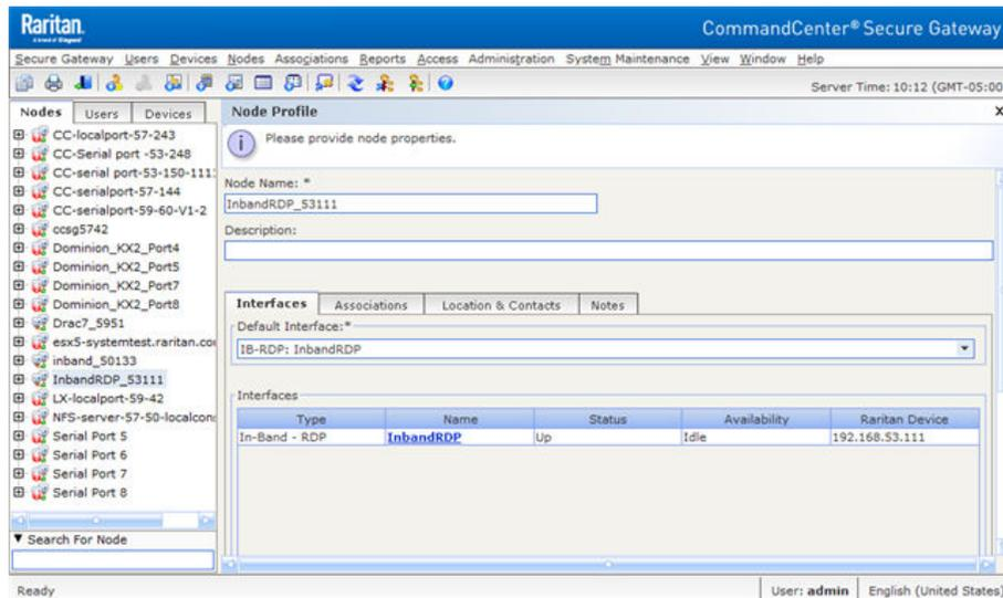
1. **Nodes tab:** Click the Nodes tab to display all nodes in a tree view. Interfaces are grouped under their parent nodes. Click + and - to expand or collapse the tree. Click a node to view the Node Profile. Right-click an interface and select Connect to connect to that interface. You can sort the nodes by Node Name (alphabetically) or Node Status (Available, Busy, Unavailable). Right-click the tree view, click Node Sorting Options, and then click By Node Name or By Node Status.
