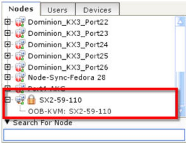
When enabled and a user disconnects from a supported node, the Admin Client shows a Lock icon on the node in the Nodes list. When locked, the same user can re-connect to the node, and the lockout time resets on disconnection.
