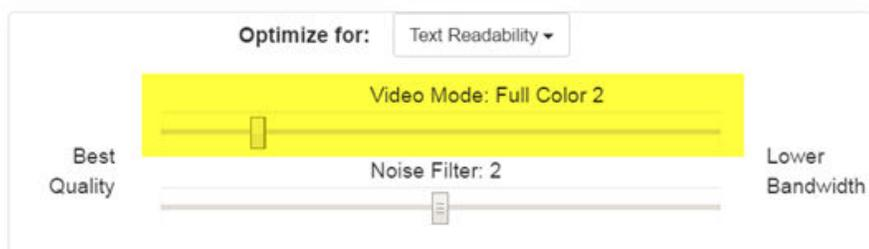
In general, moving the slider to the left results in higher quality at the cost of higher bandwidth and, in some cases, lower frame rate.
