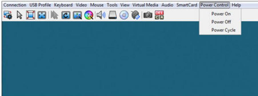
The menu option is disabled if you do not have permission for power control, and when outlets are not associated with the port.
