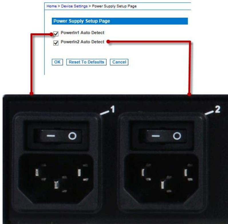
2. If you are plugging power input into power supply number one (left-most power supply at the back of the unit), then select the PowerIn1 Auto Detect option.
