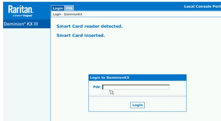
4. After successful entry of the card's PIN, access is granted if the card contains an authentication certificate approved by Client Certificate Authentication. See **Client Certificate Authentication Settings** (on page 190).
