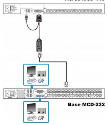
Warning: If any 2nd-tier switch is a dual-user MCD model, DO NOT connect a keyboard, mouse and monitor to Console 2 because Console 2 is disabled.
