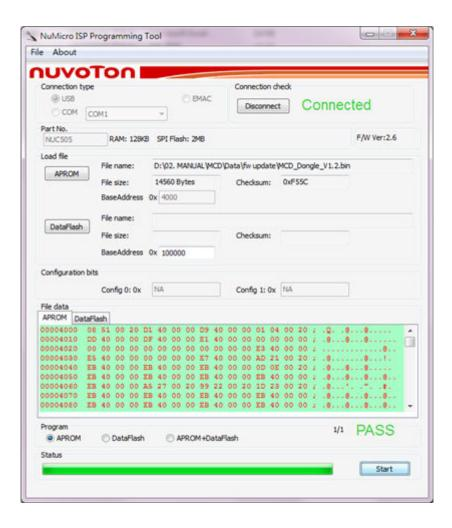
8. If there are more MDCIMs or MDUTP cables to upgrade, keep the utility open, remove the currently-connected MDCIM/MDUTP and reconnect a new one to the computer. Then repeat steps 6 to 8 until all MDCIMs and MDUTP cables are upgraded.
