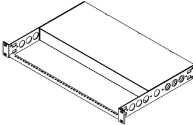
4. Fasten the rackmount brackets' ears to the rack using your own fasteners.
