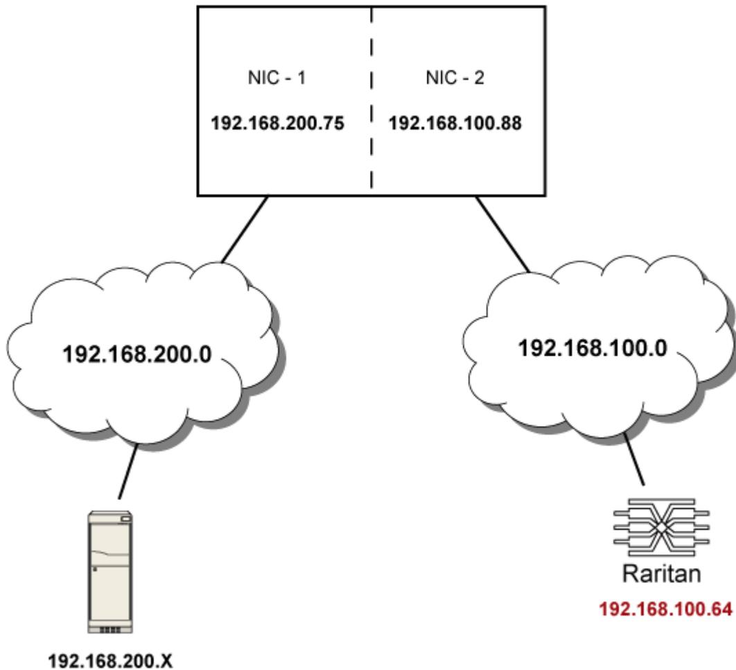
In this example, NIC-2 (192.168.100.88) is the next hop router for your PX2 to communicate with any device in the other subnet 192.168.200.0.
