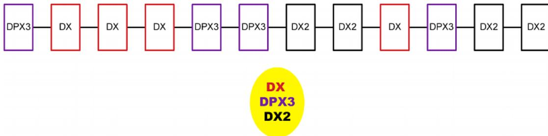
You can add a DPX2 sensor package to the end of such a sensor-mixing chain if needed. See *Connecting a DPX2 Sensor Package to DX2, DX or DPX3* (on page 40).
