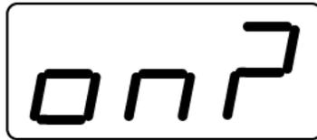
3. Press and hold the Up button until the above confirmation message disappears, indicating that the outlet has been turned on.
