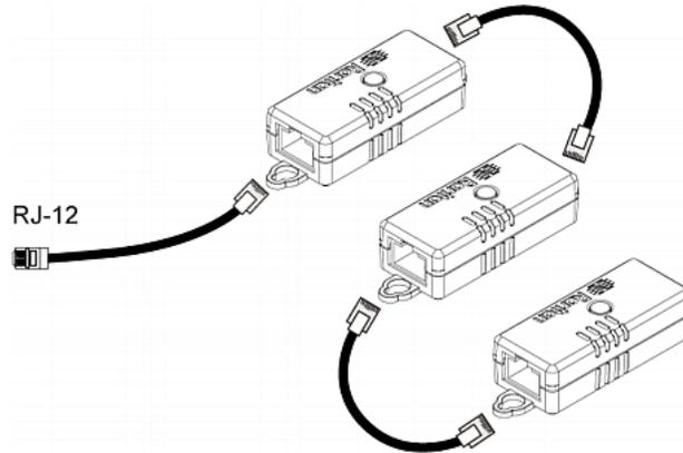
3. Connect the first DPX3 sensor package to the PX2.
