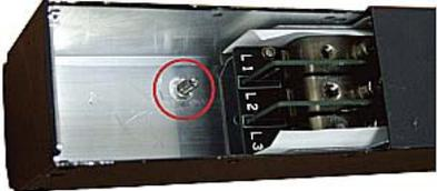
For in-line monitors, make sure to identify the inlet terminal blocks (rear of monitor) and outlet terminal blocks (front of monitor). Each inlet terminal block has a corresponding outlet terminal block.
