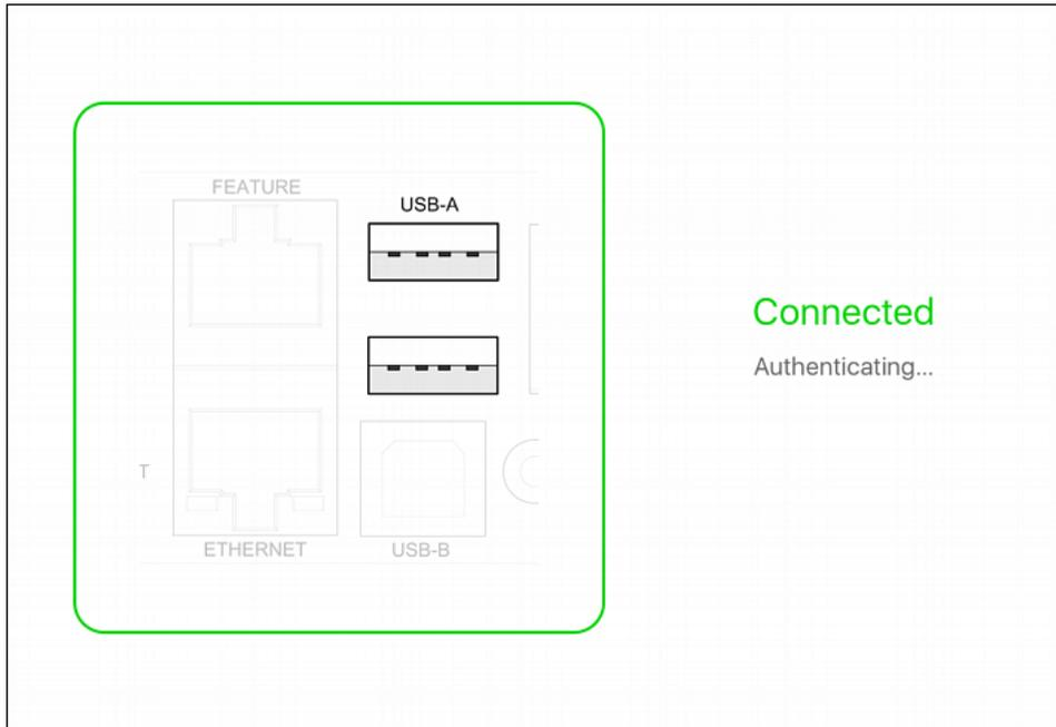
2. If the factory-default user credentials "admin/raritan" remain unchanged, PDView automatically logs in to the web interface of PX2. If they have been changed, the login screen displays instead and you must enter appropriate user credentials for login.
