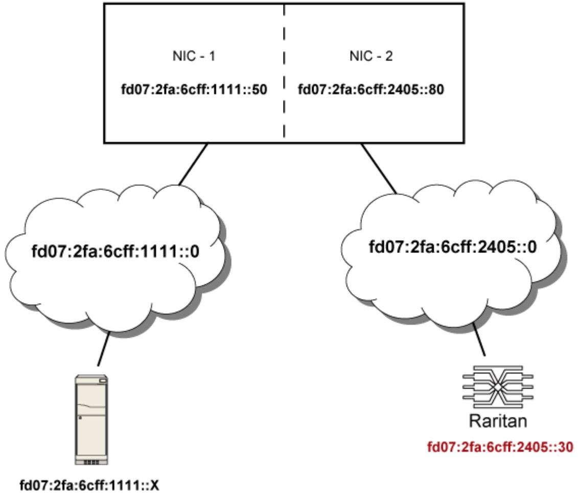
In this example, NIC-2 (fd07:2fa:6cff:2405::80) is the next hop router for your PX2 to communicate with any device in the other subnet fd07:2fa:6cff:1111::0.
