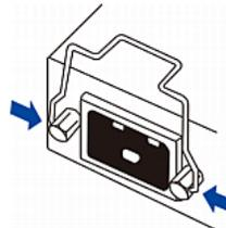
3. Connect the power cord to the inlet, and press the clip toward the power cord until it holds the cord firmly.
