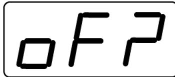
3. Press and hold the Down button until the above confirmation message disappears, indicating that the outlet has been turned off.
