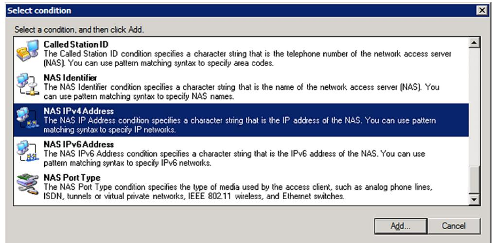
6. The NAS IPv4 Address dialog appears. Type the PX2 IP address -- *192.168.56.29*, and click OK.
