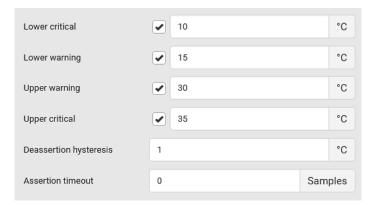
For concepts of thresholds, deassertion hysteresis and assertion timeout, see *Sensor Threshold Settings* (on page 777).
