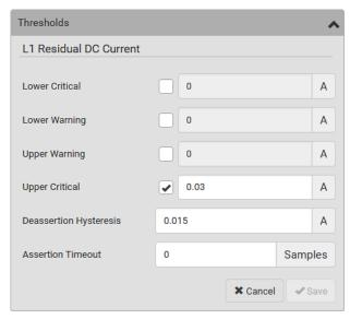
For concepts of thresholds, deassertion hysteresis and assertion timeout, see *Sensor Threshold Settings* (on page 777).
