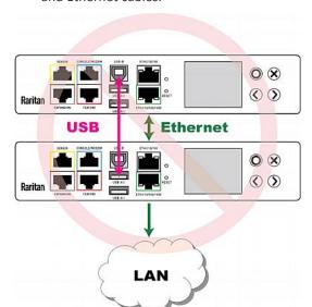
One device is connected to another device via two cascading cables - USB and Ethernet cables.
