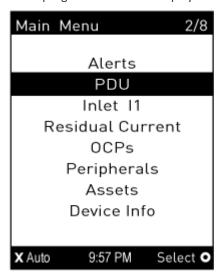
If any alerts exist, the top and bottom bars on the LCD display change the color from black to yellow or red. See *Operating the Dot-Matrix LCD Display* (on page 123).
