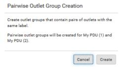
3. Pairwise outlet groups are created and named automatically for all outlets on the master and link unit, such as "Outlet pair 1", "Outlet pair 2", "Outlet pair 3", etc.
