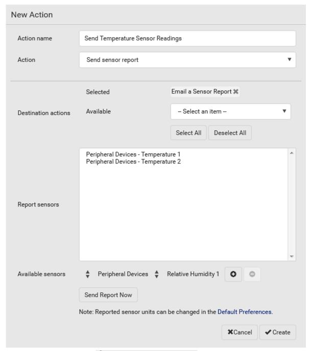
3. Click New Scheduled Action to create a timer for performing the 'Send Temperature Sensor Readings' action hourly. For details, see *Scheduling an Action* (on page 354).
