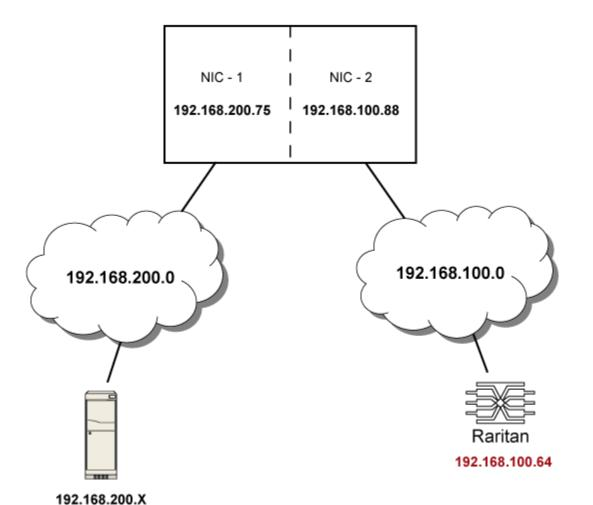
In this example, NIC-2 (192.168.100.88) is the next hop router for your PX3 to communicate with any device in the other subnet 192.168.200.0.
