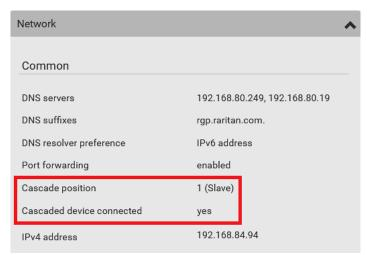
The final slave device shows a non-zero number which indicates its
