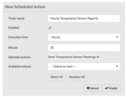
Then the PX3 will send out an email containing the specified temperature sensor readings hourly every day.
