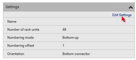
2. Make changes to the settings by directly typing a new value, or clicking that field to select a different option.
