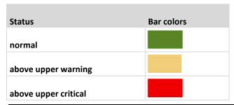
Note: The "below lower warning" and "below lower critical" states also show yellow and red colors respectively. However, it is not meaningful to enable the two thresholds for current levels.
