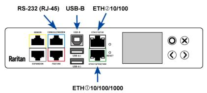
To use the command line interface (CLI) for configuration, establish an RS-232 or USB connection.
