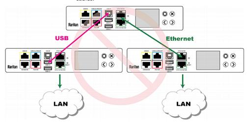
One cascaded device has two downstream devices.
