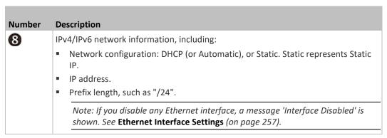
If you do not enable IPv4/IPv6 settings, an 'IPv4 (or IPv6) Disabled' message is displayed.
