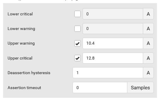
For concepts of thresholds, deassertion hysteresis and assertion timeout, see *Sensor Threshold Settings* (on page 777).
