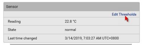
Tip: The date and time shown on the PX3 web interface are automatically converted to your computer's time zone. To avoid time confusion, it is suggested to apply the same time zone settings as those of PX3 to your computer or mobile device.
