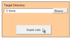
Verify that at least 3 configuration files are created - fwupdate.cfg, config.txt and devices.csv. You are ready to configure or upgrade any PX3 with these files.
