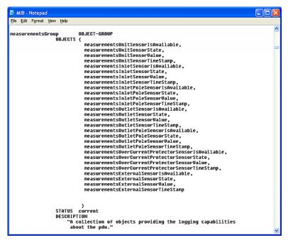
For example, the measurementsGroup group contains objects for sensor readings of PX3 as a whole. One object listed under this group, measurementsUnitSensorValue, is described later in the MIB as "The sensor value". pduRatedCurrent, part of the configGroup group, describes the PDU current rating.
