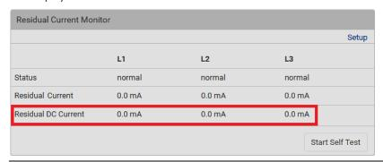
Note: To determine the RCM's normal, warning and critical levels, configure the RCM current thresholds. See **Setting RCM Current Thresholds** (on page 692). To configure the residual DC current thresholds, see **Setting RCM DC Current Thresholds** (on page 694).
