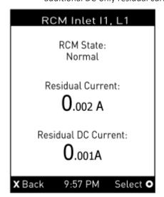
If your PX3 has more than one inlet, a list of inlets is displayed, along with each inlet's RCM state and reading(s).
