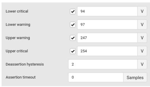
For concepts of thresholds, deassertion hysteresis and assertion timeout, see *Sensor Threshold Settings* (on page 777).
