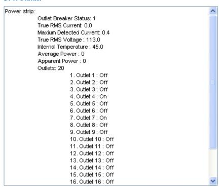
2. A status box appears, displaying details of the controlled PX3, including power state of each outlet on the device.
