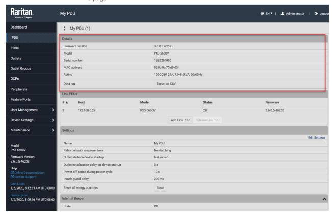
The PDU page displays the following information about the master PDU:
