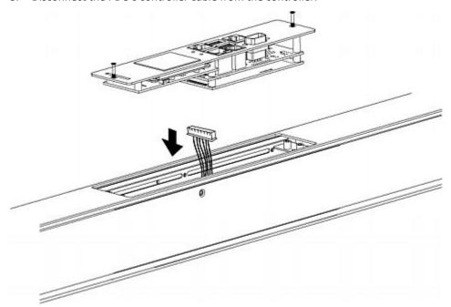
Get a new PX3 controller and install it back into the PDU in the reverse order.
