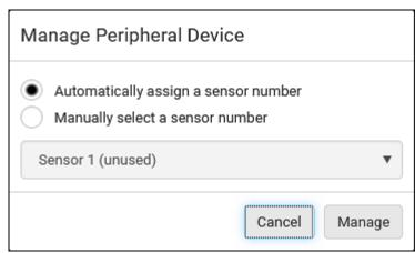
To let PX3 randomly assign an ID number to it, select "Automatically assign a sensor number."
