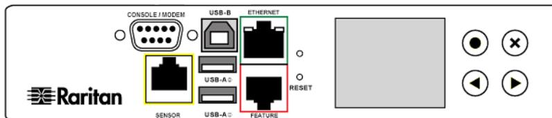
The operation of its front panel button is similar to the front panel operation of PX3 with iX7™ controller (PX3-iX7). See **Operating the Dot-Matrix LCD Display** (on page 123).
