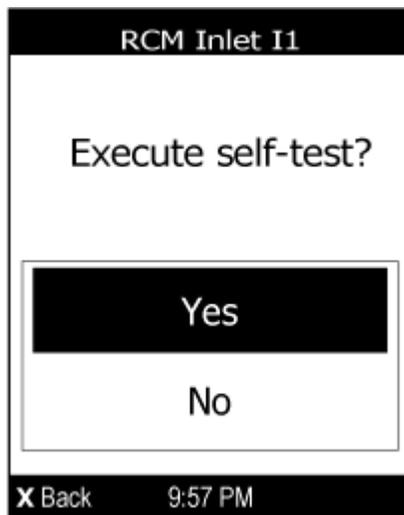
6. After completing the RCM self-test, the LCD display indicates the RCM self-test result: passed or failed.
