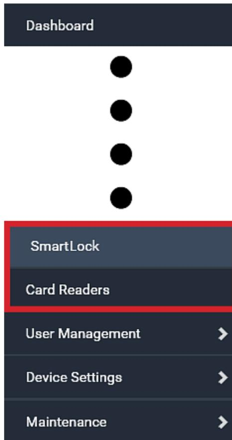
Note that "SmartLock" appears only when your door handles are connected to PX3 via **DX2-DH2C2**, but "Card Readers" appears as long as PX3 detects the presence of any card reader -- either a standalone USB card reader or a card reader integrated with the door handles.
