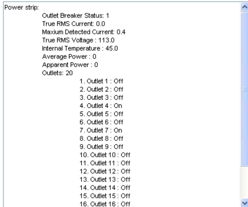
2. A status box appears, displaying details of the controlled PX3, including power state of each outlet on the device.
