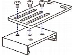
5. Using rack screws, fasten the PX3 device to the rack through the claw-foot brackets.
