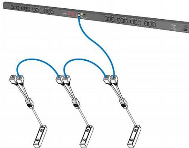
5. Repeat Step 3 to connect IT devices to the other composite asset strips in the chain.
