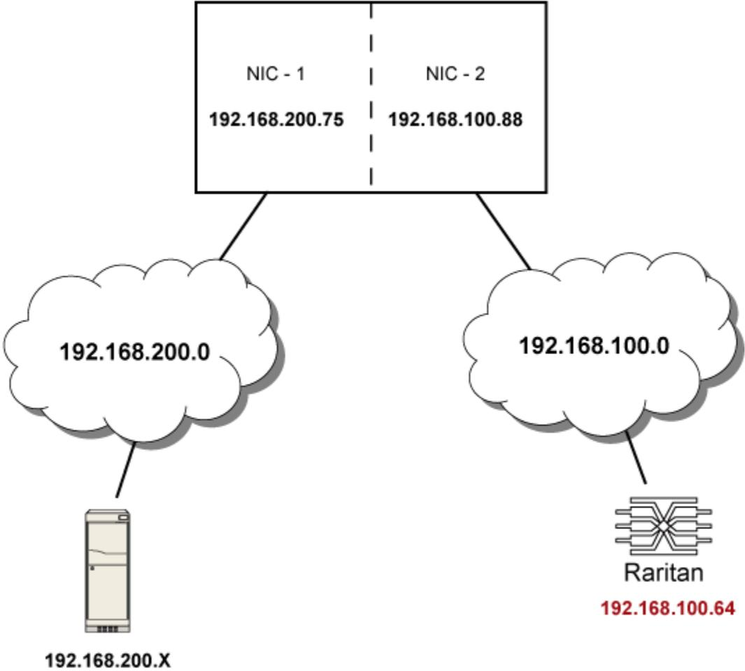
In this example, NIC-2 (192.168.100.88) is the next hop router for your PX3 to communicate with any device in the other subnet 192.168.200.0.
