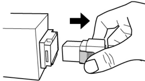
▶ **To disconnect a line cord with slide release buttons:**
