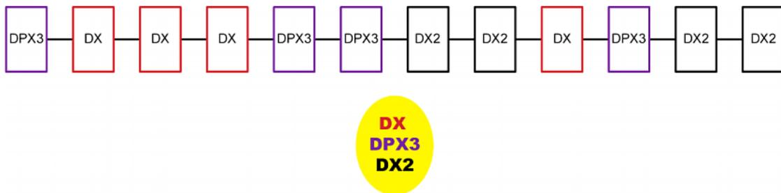
You can add a DPX2 sensor package to the end of such a sensor-mixing chain if needed. See **Connecting a DPX2 Sensor Package to DX2, DX or DPX3** (on page 56).
