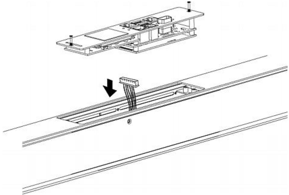
4. Get a new PX3 controller and install it back into the PDU in the reverse order.
