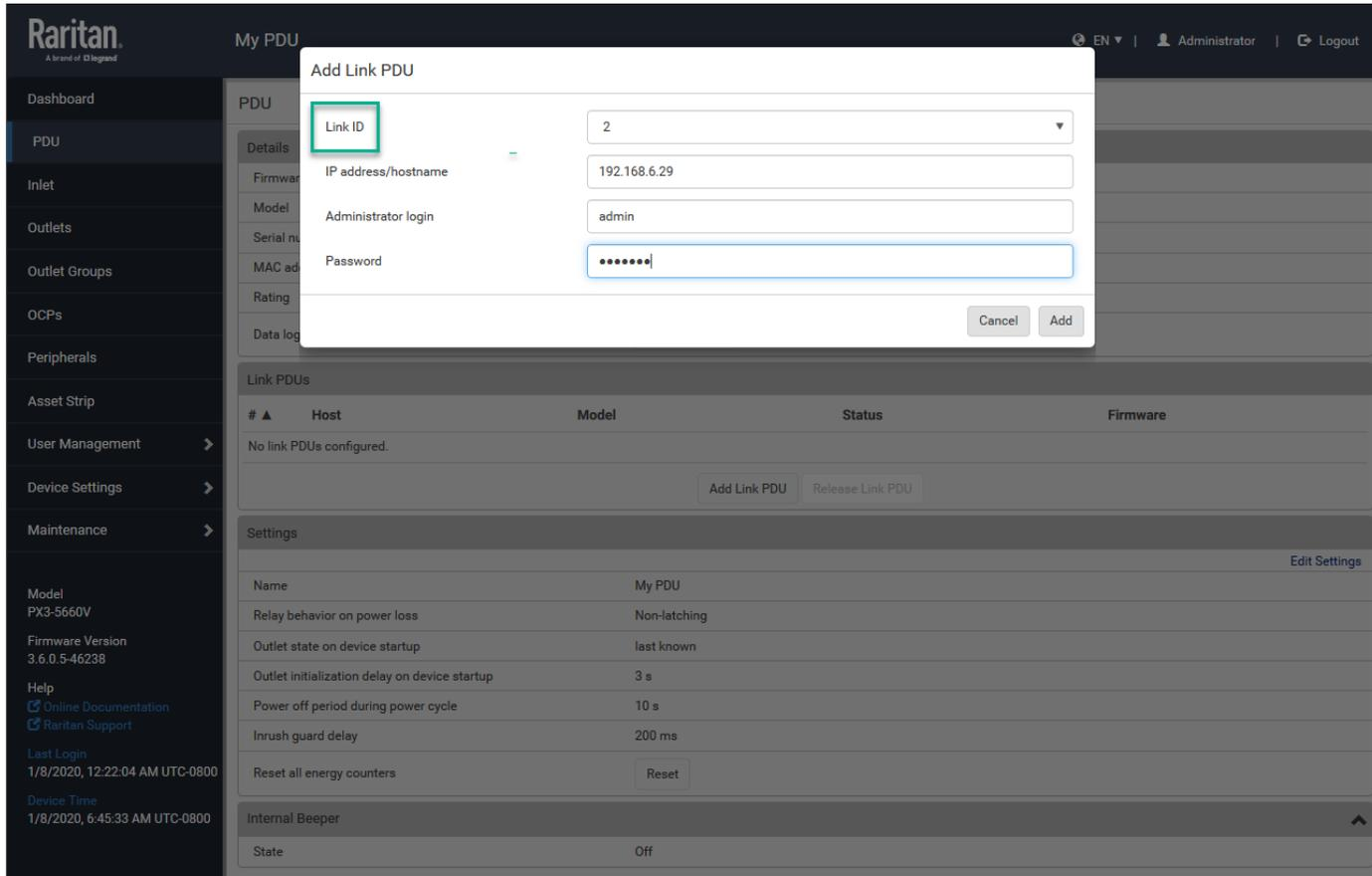
1. The Link ID is populated as the next available ID number (2-8), assigned sequentially as each link unit is added to the chain to identify the link unit in the user interfaces. Note: From the drop-down, you can manually select the desired Link ID to order the link units in the chain as desired. Once associated with a link unit, the Link ID cannot be edited.
