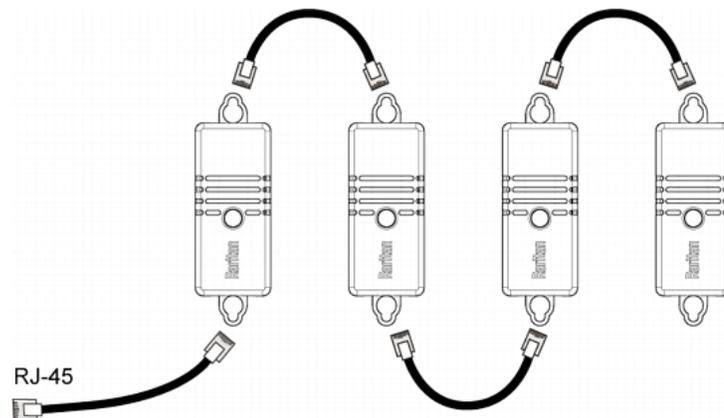
3. Connect the first DX2 sensor package to the PX3 by plugging its cable's connector into the RJ-45 SENSOR port of the PX3.
