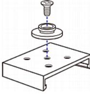
4. Align the large mounting buttons with the mounting holes in the cabinet, fixing one in place and adjusting the other.
