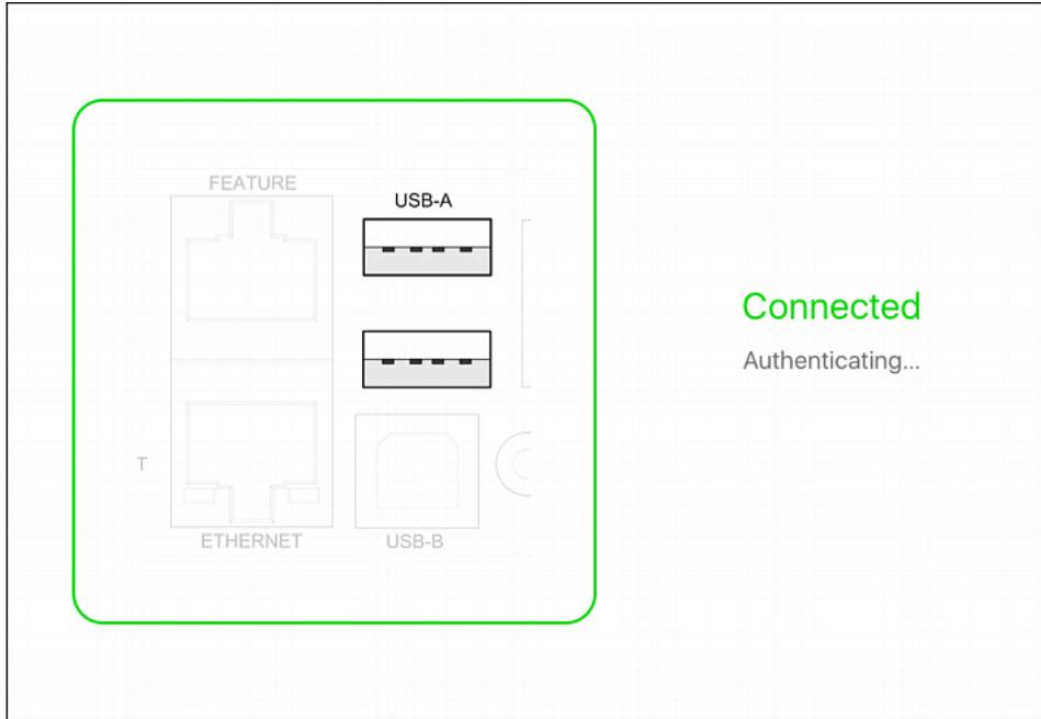
2. If the factory-default user credentials "admin/raritan" remain unchanged, PDView automatically logs in to the web interface of PX3. If they have been changed, the login screen displays instead and you must enter appropriate user credentials for login.
