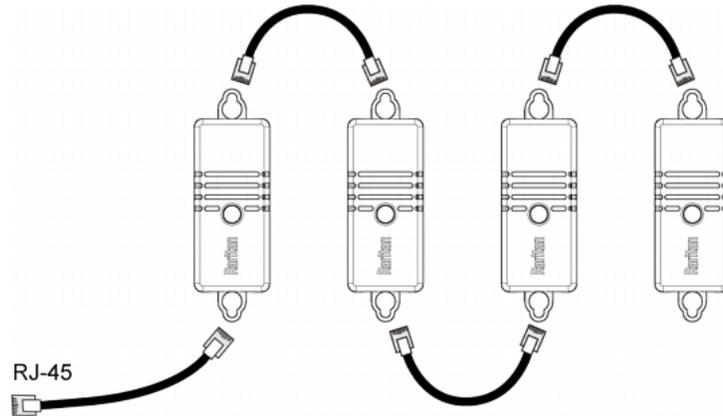
3. Connect the first DPX3 sensor package to the PX3 by plugging its cable's connector into the RJ-45 SENSOR port of the PX3.
