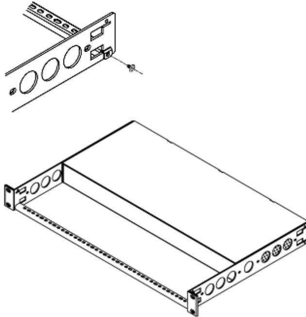
4. Fasten the rackmount brackets' ears to the rack using your own fasteners.
