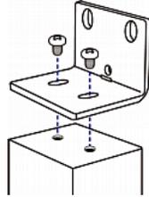
3. Repeat Steps 1 to 2 to screw another L-bracket to the bottom of the device.
