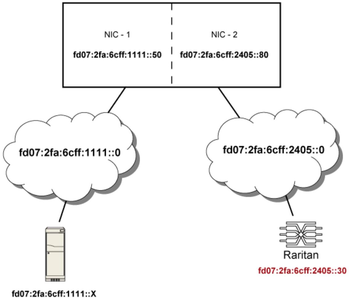
In this example, NIC-2 (fd07:2fa:6cff:2405::80) is the next hop router for your PX3 to communicate with any device in the other subnet fd07:2fa:6cff:1111::0.
