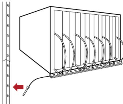
6. Repeat the above steps to connect additional blade extension strips. Up to 128 asset tags on blade extension strips are supported per FEATURE port.
