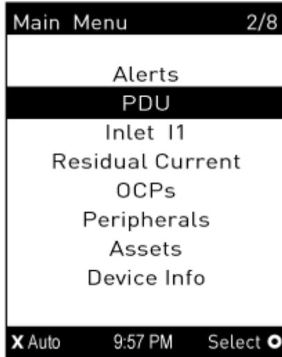
If any alerts exist, the top and bottom bars on the LCD display change the color from black to yellow or red. See **Operating the Dot-Matrix LCD Display** (on page 123).
