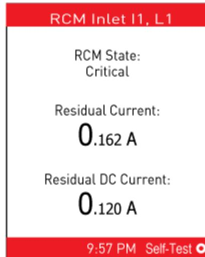
If your PX3 has more than one inlet, only the inlet which has the RCM alarm enters the critical state.
