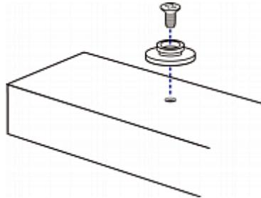
4. Screw a button in the screw hole near the top. The recommended torque for the button is 1.96 N·m (20 kgf·cm).
