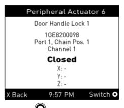
Press  $oldsymbol{O}$  to turn on or off the actuator. A confirmation message similar 2. to the following is shown.
