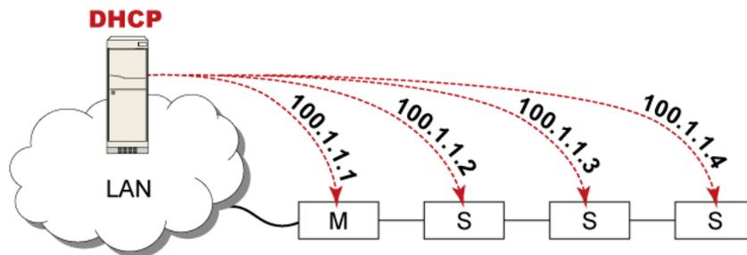
In this mode, the DHCP server communicates with every cascaded device respectively and assigns four *different* IP addresses. Each device has its own IP address.
