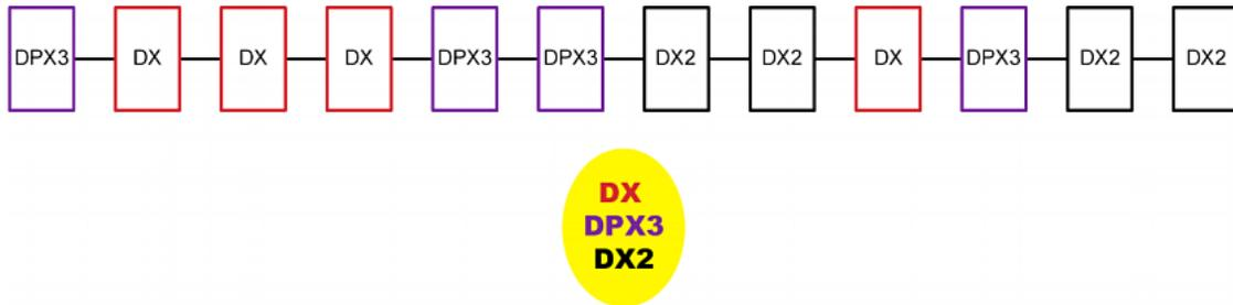
You can add a DPX2 sensor package to the end of such a sensor-mixing chain if needed. See *Connecting a DPX2 Sensor Package to DX2, DX or DPX3* (on page 46).
