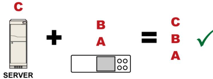
In reality some servers may provide a partial (or even a full) certificate chain instead of a single server certificate. If your server provides a partial certificate chain containing 'Certificate B' and 'Certificate C', then you only need to upload 'Certificate A' to the receiver. If the server has a full certificate chain containing Certificates 'A', 'B', and 'C', then you also need to upload the root certificate 'A'.
