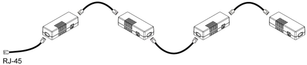
3. Connect the first DX sensor package to the PXC/PX0 by plugging its cable's connector into the RJ-45 SENSOR port of the PXC/PX0.
