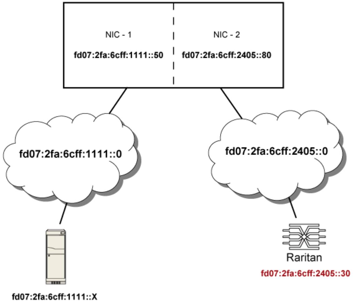
In this example, NIC-2 (fd07:2fa:6cff:2405::80) is the next hop router for your PXC/PX0 to communicate with any device in the other subnet fd07:2fa:6cff:1111::0.
