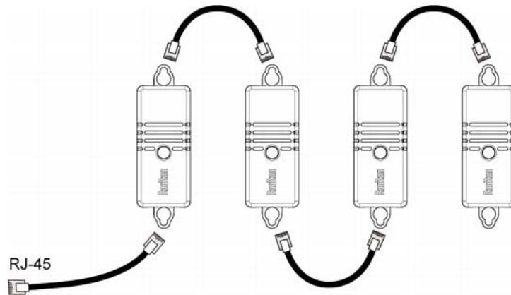
3. Connect the first DPX3 sensor package to the PXC/PX0 by plugging its cable's connector into the RJ-45 SENSOR port of the PXC/PX0.
