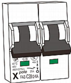
3. Examine your PXC/PXO and the connected equipment to remove or resolve the cause that results in the overload or short circuit. **This step is required, or you cannot proceed with the next step.**
