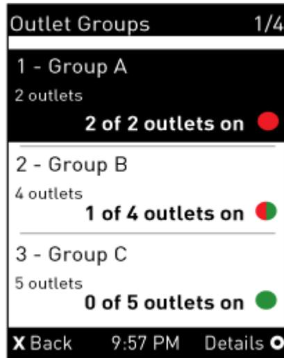
The currently-selected outlet group's number and total of outlet groups are indicated in the top-right corner of the display, such as "1/4" in the above diagram.
