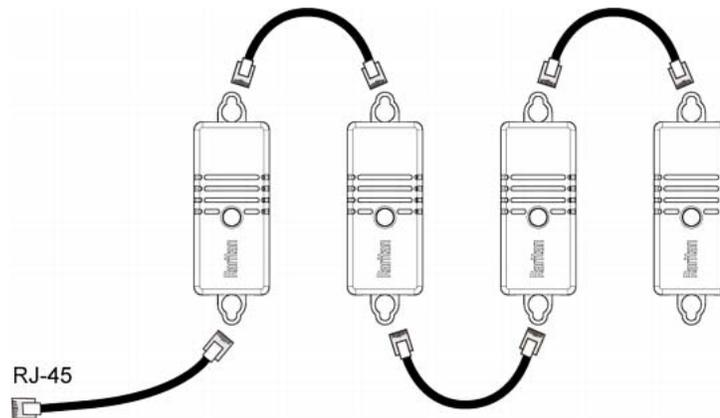
3. Connect the first DX2 sensor package to the PXC/PX0 by plugging its cable's connector into the RJ-45 SENSOR port of the PXC/PX0.
