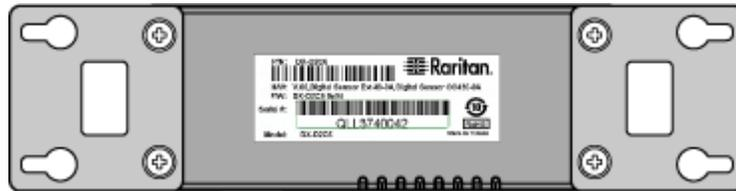
The serial number for each sensor or actuator appears listed in the web interface after each sensor or actuator is detected by the PXC/PX0. Match the serial number from the tag to those listed in the sensor table.
