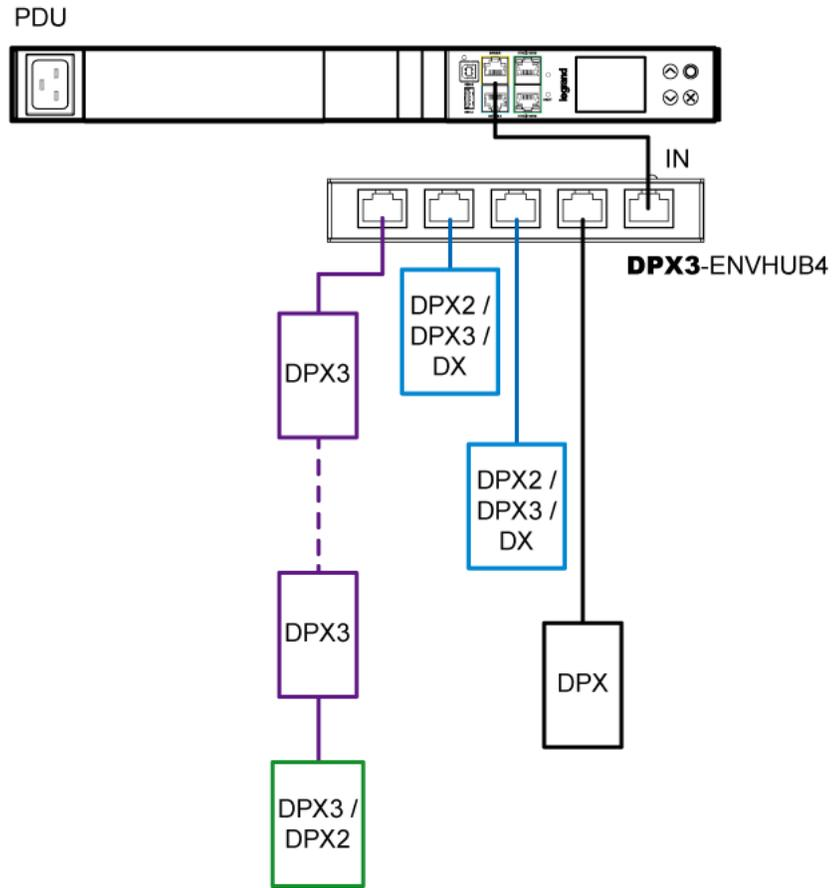
► **Mix DX2, DX and DPX3 in a sensor chain:**
