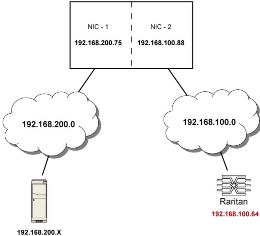
In this example, NIC-2 (192.168.100.88) is the next hop router for your PXC/PX0 to communicate with any device in the other subnet 192.168.200.0.
