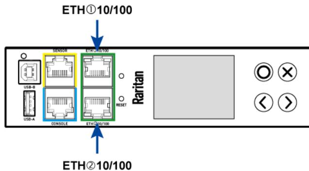
Warning: Accidentally plugging an RS-232 RJ-45 connector into the Ethernet port can cause permanent damage(s) to the Ethernet hardware.
