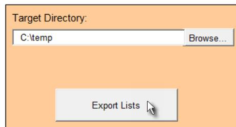
6. Verify that at least 3 configuration files are created - *fwupdate.cfg*, *config.txt* and *devices.csv*. You are ready to configure or upgrade any PXC/PXO with these files. See ***Configuration or Firmware Upgrade with a USB Drive*** (on page 601).
