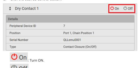
2. Confirm the operation on the confirmation message. An actuator's state is marked in red when it is turned on.
