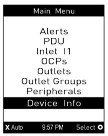
If any alerts exist, the top and bottom bars on the LCD display change the color from black to yellow or red. See *Operating the Dot-Matrix LCD Display* (on page 62).
