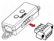
3. After connecting detectors/switches to the terminal module, plug the terminal module back into the sensor box, and then tighten the screws at two sides of the terminal module.
