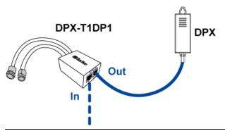
Note: You CANNOT cascade more than two sensor packages in this DPX sensor chain.
