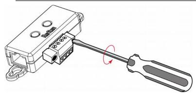
2. Separate the terminal module from the sensor box.
