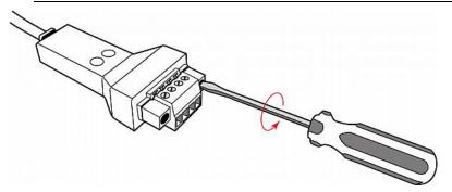
2. Separate the terminal module from the sensor box.
