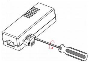
2. Separate the terminal module from the sensor box.
