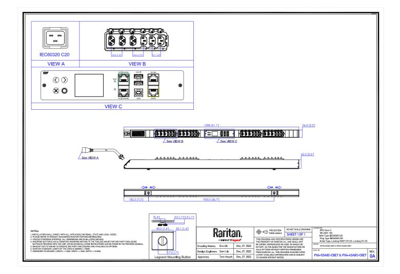
Technical Specifications Model Number: PX4-53A8C-C8E7A0 100-240V, 1Φ, 16/16A, 1.6-3.8kVA
